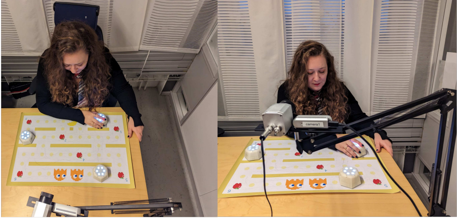
Fig. 1 Setup for data collection. Left: A top view showing the game setup, three robots on the map: One is manipulated by the user and two others chase the users autonomously. Right: A front view showing the thermal camera on the left and RGB camera on the right.
